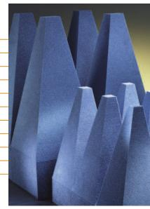
The SFC-EM products are optimized for low frequency performance. C-RAM SFC-EM are truncated to save space and yield a rugged product. Ideal for MIL SPEC 462 — C, D, and E and CISPR-25 chambers. Also a low cost solution for EN 1000-4-3 and derivative specifications from 80 MHz through 40 GHz.
