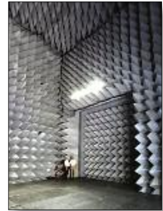
The Lockheed Martin Newtown chamber is an extremely "quiet" PIM test facility.
