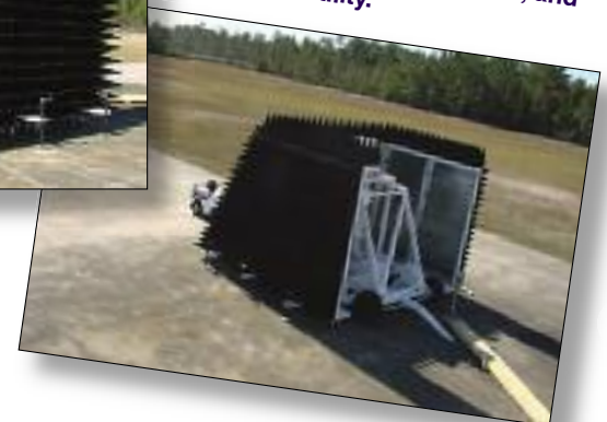
C-RAM ODP on a portable framework makes for an unusual radar absorber system.
