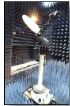
Powerful antenna systems can be tested in the CIARS anechoic chamber.
